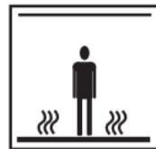
Flexible sheet heating units are installed within the floor. **DO NOT** penetrate with nails, screws, or similar devices. **DO NOT** restrict the thermal emission of the heated floor. **DO NOT** affix materials other than those recommended
